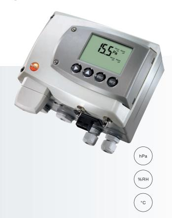
The differential pressure transmitter testo 6351 was developed specially for monitoring differential pressure in the measuring range from 50 Pa to 2000 hPa. In cleanroom technology, the maintenance of positive pressure prevents the entry of contaminated air. In addition to this, the flow velocity or the volume flow can be calculated from the measurement of the differential pressure in a Pitot tube.
